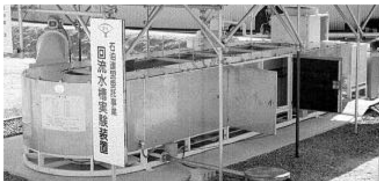
Figure 1 Circulating Water Channel
