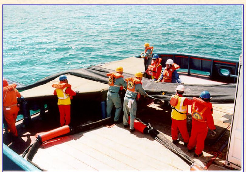
Boom is deployed while being inflated
